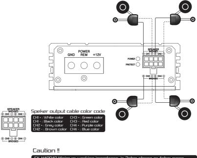
SK-M4004D Minimum working impedance is 20hm stereo or 40hm mono. Impedance lower than 20hm stereo or 40hm mono can damage the amplifier
