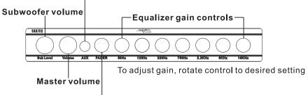
**Fader control:** Use to balance sound between front and rear speakers
